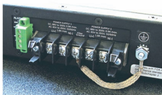
FIGURE 7: Power connection and alarm contacts
